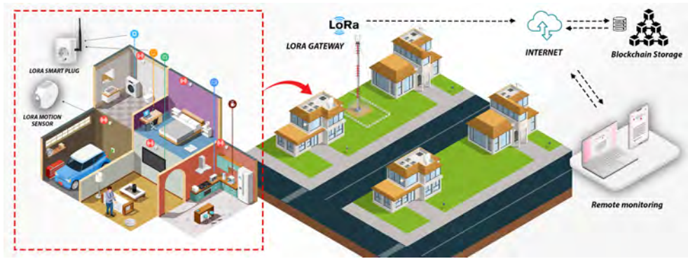
Figure 5.30: General scheme of the LoRa monitoring system
