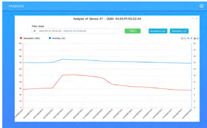
Figure 5.5: Web application device dashboard page showing the chart of moisture and resistance in function of time, the user can filter data by date and download it as Excel or CSV file.
