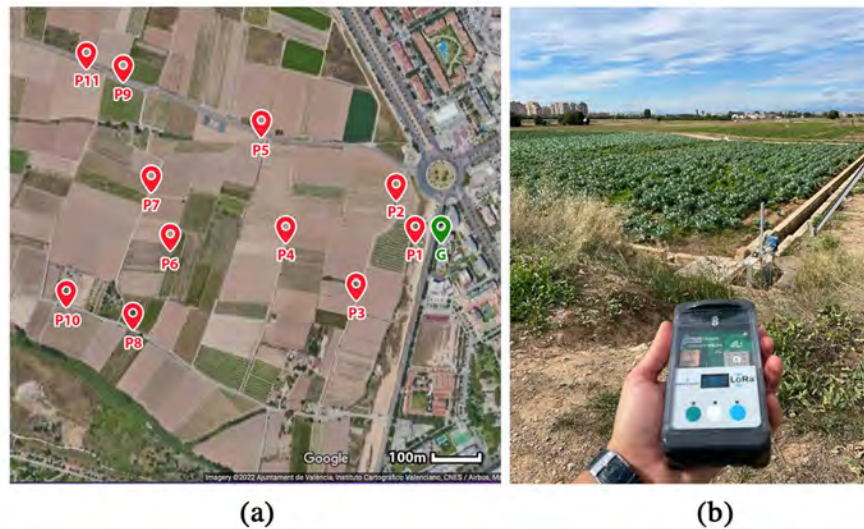
Figure 5.21: Experimental setup for outdoor LoRa communication test. (a): P1 to P14 represent the measurement locations, G represent the gateway location. (b): LoRa Mote II used as LoRa end-node [244].
