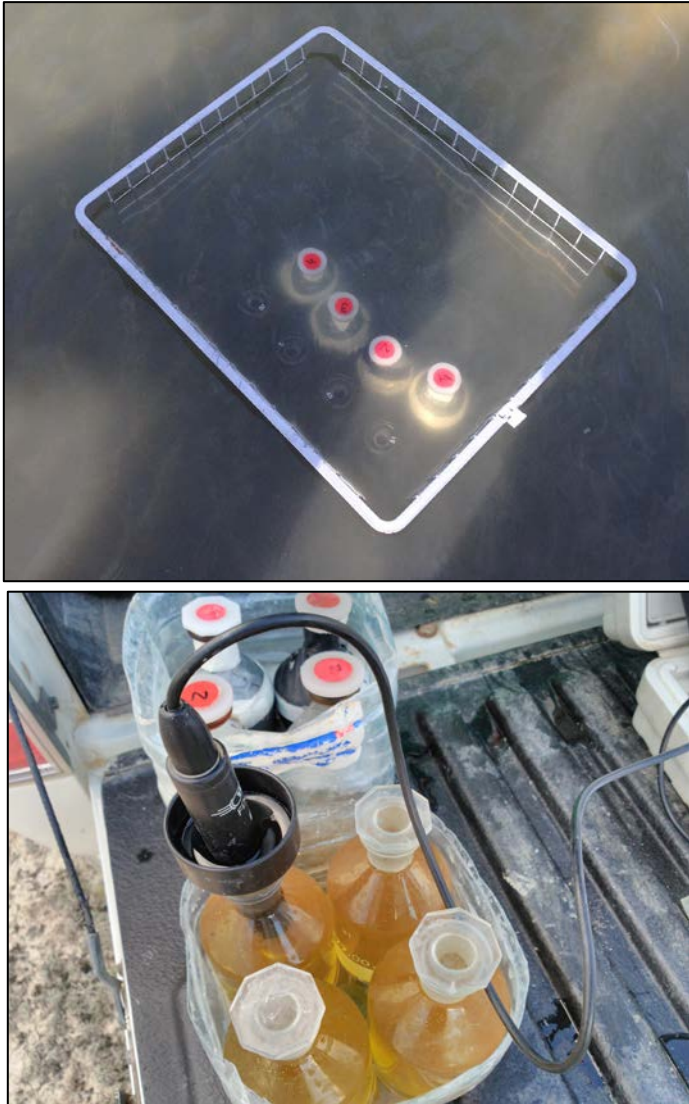
Figure 2.6. Winkler bottles for measuring planktonic metabolic rates (dark and light bottles). The water samples were submerged to perform incubations at the in-situ light and temperature conditions.
