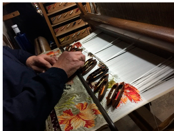
Figure 1. Making a Valencian espolín with a Jacquard loom. It can be seen how the golden threads do not go from side to side of the fabric but remain concentrated around the pictorial motifs.
