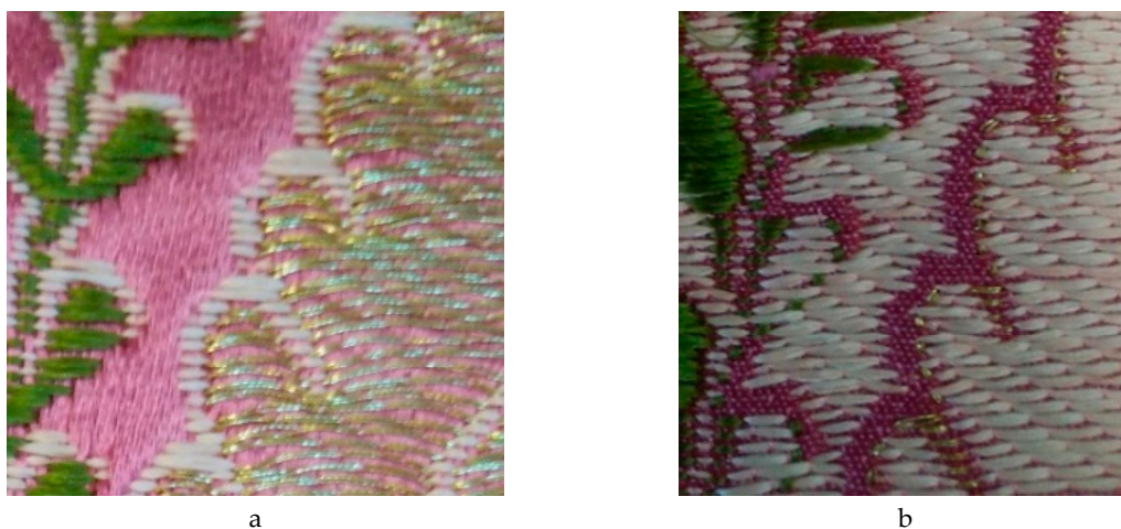
Figure 7. Example of a textile where one of the threads of the pictorial part overlays the background from the backside and also is interlaced from time to time with the warp threads, where: (a) front side; (b) backside (note that this image has been mirrored for an easy comparison).
