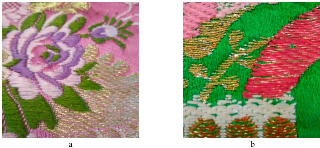
Figure 5. Examples of textiles seen from the front side (a,b). It can be seen that threads of different colors do not cross or overlap with others of the pictorial part.
