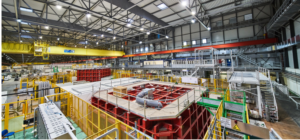
Figure 3.1: View of the Neutrino Platform. In the front of the picture the cryostat of ProtoDUNE-SP can be observed. In the left back part, the cryostat of ProtoDUNE-DP is present too. Image from [112].
