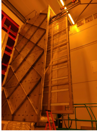
Figure 4.21: APA completely instrumented about to be tested in the cold box.
