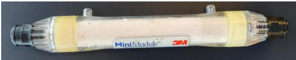
Figure 3.4. Polypropylene hollow fibre membrane contactor used in this thesis.
