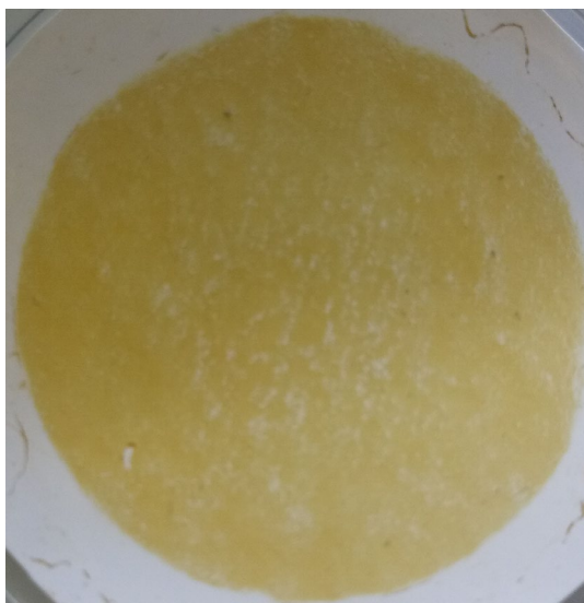
Figure S 5. Representative example of the collected solid particles onto the 0.025 \mu\text{m} filter at the end of the crystallisation tests.
