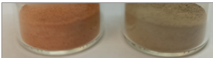
Figure 3.2.2. Colour difference between the pristine MIL-100(Fe) (left) and the final biocomposite (right) after the encapsulation process.
