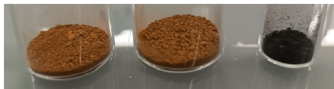
Figure 5.2.1. Image of the obtained MM-MUV-2 derivatives: MUV-2(Fe/Co) (left), MUV-2(Fe/Ni) (centre), in comparison with MUV-2(Fe) crystalline powders (right).
