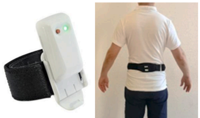
Fig. 1. Inertial measurement unit (IMU) and its location to assess posture parameters.
