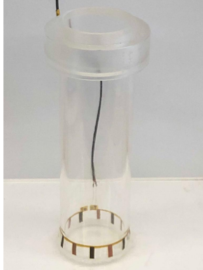
Fig. 4. Implemented sensor prototype (7 cm applicator is shown). It can be seen the two sets of six detector sections (12 strips) interspersed with each other and located 3 mm away from the bottom of the methacrylate plate. Strips are 1.5 cm height, 0.5 cm width.
