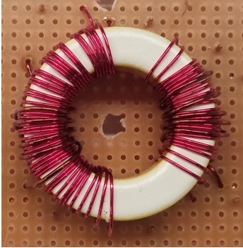
Figure 12. Five windings' coupled inductor on an iron powder core. On the left side are three well coupled windings and on the right side two well coupled windings. But these last two windings are not so well coupled to the first three ones.
